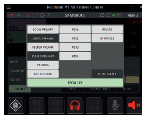
Snapshots can be saved and recalled through the Snap menu. During recall, a filter function (shown in the image) allows the selection of which parts should be loaded
