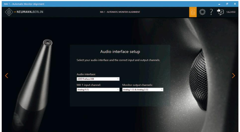
Figure 1 - The software guides through the system setup process, here showing the selection of the ASIO audio interface (Windows 10) and input/output channels
