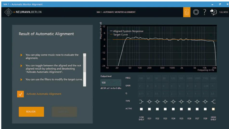
Figure 5 - Measurement result including correction at the listening position for the main listening test
