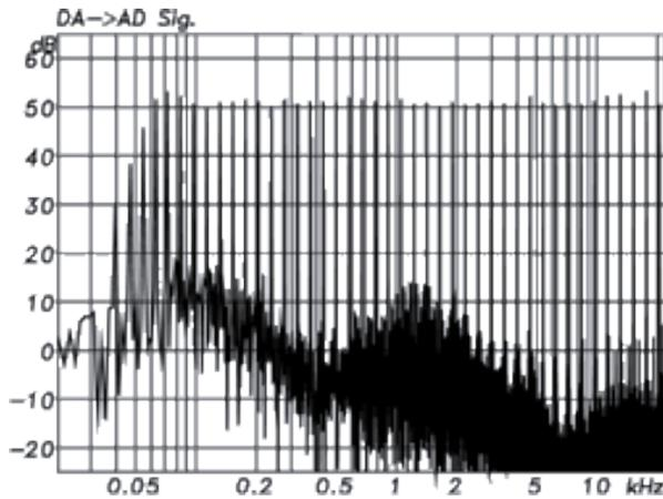
Intermodulation distortion of a two-way loudspeaker
