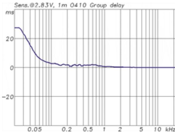
Group delay of a large three-way loudspeaker
