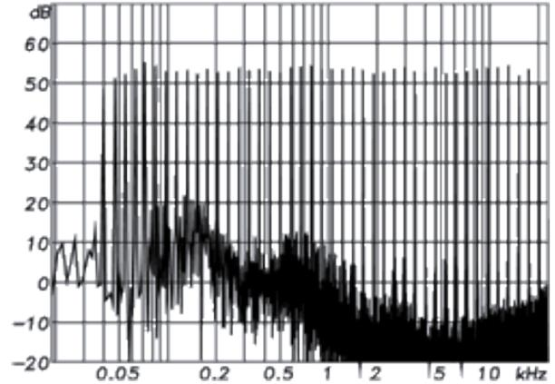
Intermodulation distortion of a three-way loudspeaker
