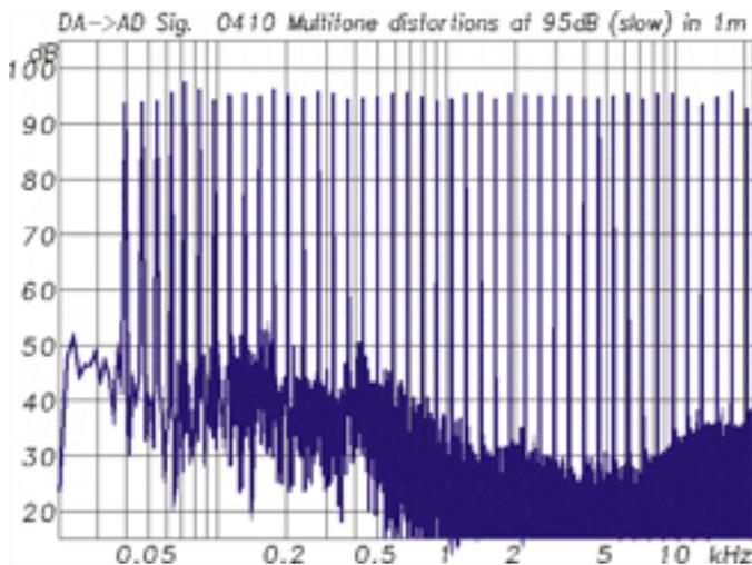
Intermodulation distortion of a large three-way loudspeaker
