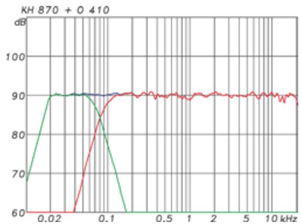
Large three-way loudspeaker with a subwoofer
