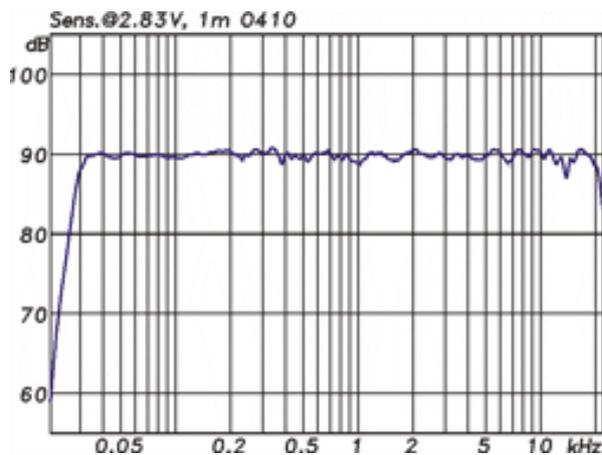
Frequency response of a large three-way loudspeaker (O 410)
