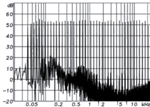
Intermodulation distortion of a three-way loudspeaker
