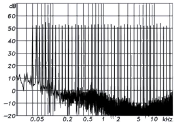
Intermodulation distortion of a three-way loudspeaker with a subwoofer
