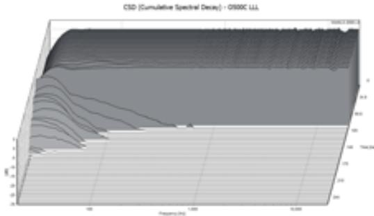
Waterfall plot of a linear-phase DSP loudspeaker
