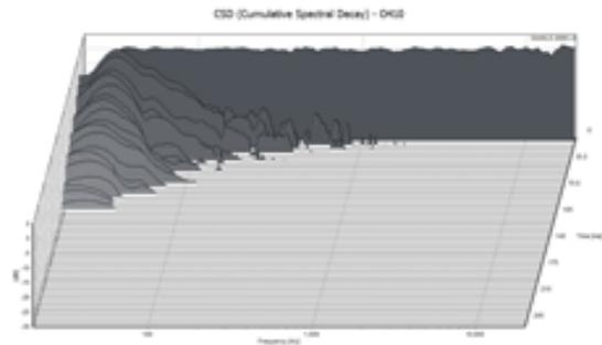
Waterfall plot of a loudspeaker with no resonances
