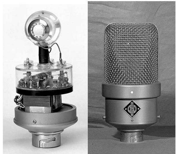
Fig. 4. The M 50 Microphone
