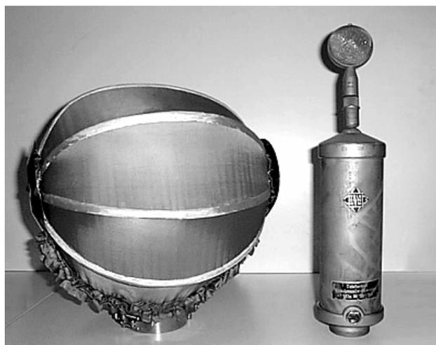
Fig. 1. CMV 3 microphone with wind shield (1930's)
