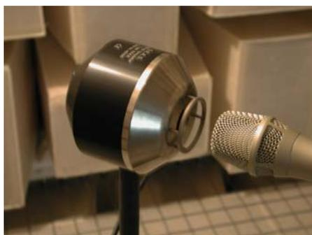
Figure 3 Artificial mouth at 0.05 m distance
