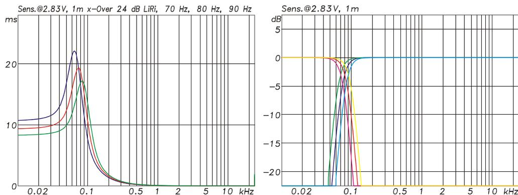
The lower the x-over frequency is the higher the group delay increase is. This leads to a less tight bass impulse.
