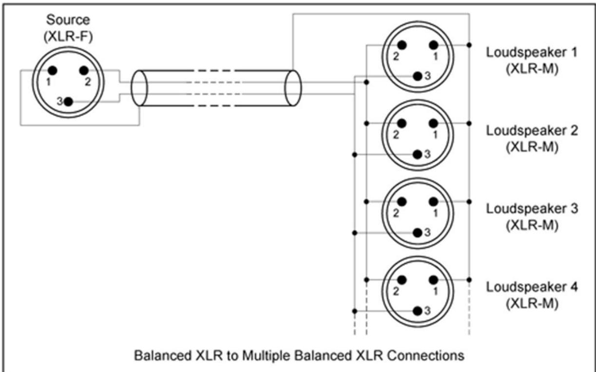
**I have no pre-amp outputs on my equipment, so how do I connect the loudspeaker to the loudspeaker outputs of my power amplifier?**
