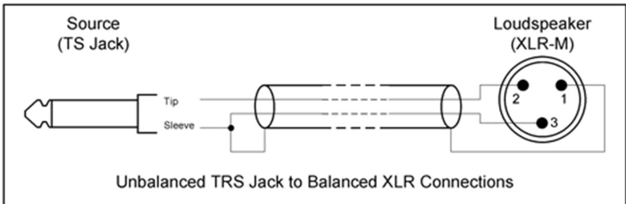
**How do I connect the stereo unbalanced output (TRS Stereo Jack) on my source equipment to the loudspeakers?**
