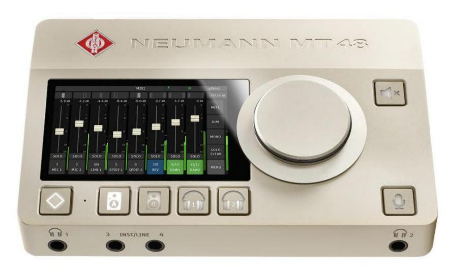
selection, and two more buttons used as headphone selectors "all configurable natively or via Neumann's desktop application". A built-in microphone is also situated on the unit's face which can be engaged by a handy talkback button. Lastly, a home button and generously sized LCD touch display are implemented in the design of the unit, rounding out its hardware UI.
