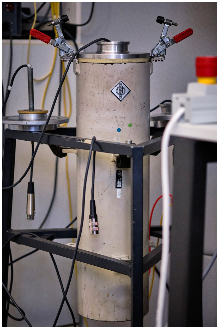
The microphone's self-noise is measured in a soundproof container ("Rauschbombe").
