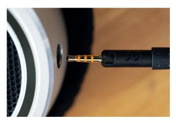
The cable of the NDH 30 is internally balanced, i.e. it has separate ground leads for the left and right earcups, which improves channel separation audibly.
