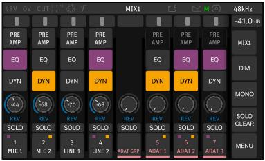
Each input channel has inserts for EQ and Dynamics processing. EQ and DYN in color indicate that processing is activated. The Analog Inputs as well as Peered Inputs also have a PREAMP page.
