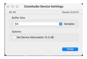
Selecting a small buffer size will give you lower latency, but it will also increase the CPU load. Selecting a larger buffer size will reduce the CPU load but results in higher latency. A good starting point is usually 64 samples. This gives you low enough latency for a direct response when you play softsynths while maintaining good CPU performance.
