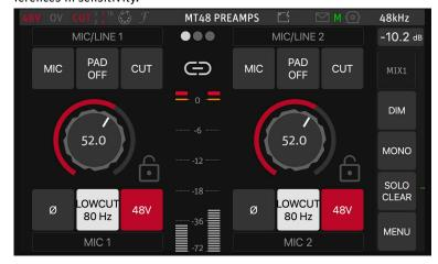
Settings can be locked by clicking on the lock symbol next to the gain knob.
