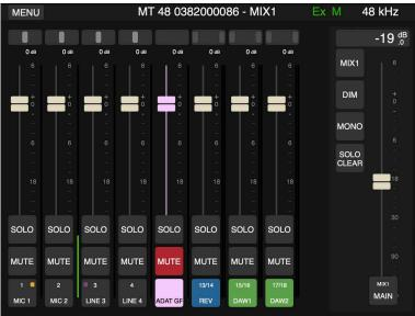
Per default, the Web Control browser page looks similar to the Remote Control App. However, the Web Control surface is optimized for touchscreen, i.e. for use with a tablet computer (see below), and it can be configured in various ways. The Web Control browser window has no size constraints so it can display more than eight channel strips.
