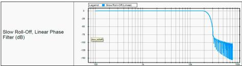
**Apodizing:** Fast roll-off, linear phase filter. Avoids pre-ringing for super accurate transient response. Latency of 35 samples.
