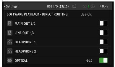
4. In the MT 48 Mixer, remove the ADAT Input channels. Go to MENU → STRIPS SETUP and disable all ADAT channels and clear the ADAT Group.
