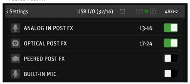
Having this option on separate driver channels allows you to record the same source with and without processing at the same time, if you wish. That way you can use the on-board processing for creative sound shaping and record a raw backup on a separate track, in case you decide otherwise.
