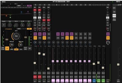
The Preamps section has additional functions not found on the hardware unit or the Remote Control app. These additional functions are especially useful in larger setups with many preamp channels. Instead of the PREAMP LINK feature, the Web Control features up to eight PREAMP LINK GROUPS (PLG) which the preamp channels can be assigned to. This allows you to control gain, polarity, low cut and cut (mute) on two or more channels simultaneously.
