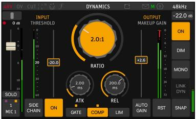
The compressor section has the following parameters:
