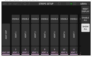
Here you can disable channel strips or enable channel strips that are currently hidden (disabled). If you enable more strips than the screen can display (eight), you can reach the additional channels by swiping.
