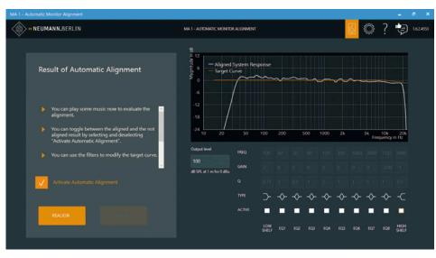
Figure 5 - Measurement result including correction at the listening position for the main listening test
