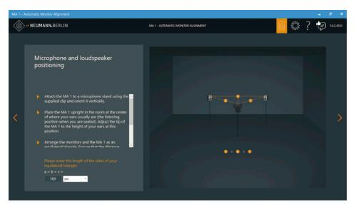
Figure 3 - The positioning of the measurement microphone at various points around the listening position is ,moderated' by the software
