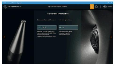
Figure 2 - Each Neumann measurement microphone has a calibration profile that is identified and loaded for measurement based on its serial and code number
