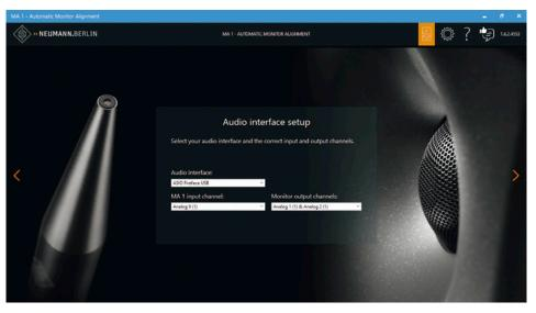
Figure 1 - The software guides through the system setup process, here showing the selection of the ASIO audio interface (Windows 10) and input/output channels
