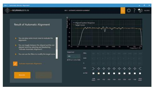
Figure 4 - Result of a test measurement that can be adjusted with a multiband EQ
